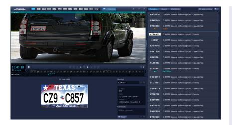
SecurOS<sup>TM</sup> Auto is an intelligent video analytics module for the SecurOS<sup>TM</sup> Premium and Enterprise video management platforms, which provides license plate recognition and comparative analysis for all types of vehicles. SecurOS<sup>TM</sup> Auto works in a wide range of internal/external conditions and delivers industry leading recognition accuracy for US and international plates.
